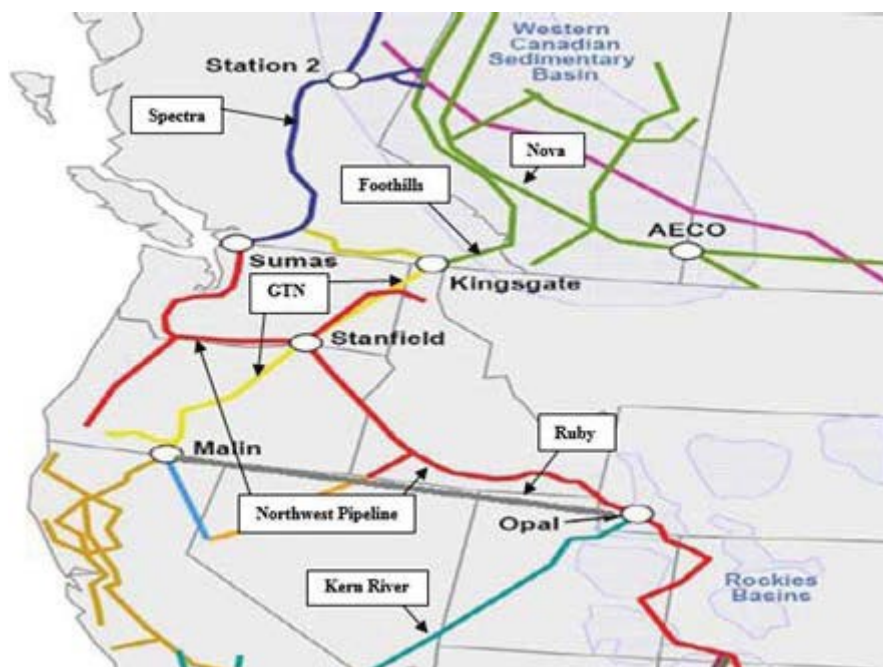
Figure 28: Pacific Northwest Pipelines Map
